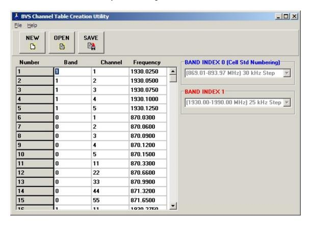
You can enter up to 30 different channels or frequencies. You can modify an existing table or create a new table by pressing the associated buttons.
